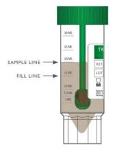
Add 5g of sample to the vial, bringing the level to the sample line.
